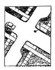
safety. Another road narrowing technique can be found by the use of medians. In one community in Maryland, medians 20 to 50 feet or more in length have been constructed in advance of intersections. It was found to effectively reduce speeds though, it was necessary to construct bulb-outs to force drivers to shift over inconveniently. Once implemented, the 85<sup>th</sup> percentile speeds were reduced by 2-5 mph.
