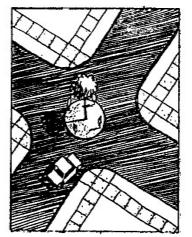
A traffic island is a defined area, painted or raised, included in highway design for the primary purposes of controlling and directing traffic movements. They also provide refuge for pedestrians, reduce excessive pavement areas, and can be used to indicate proper use of an intersection or to locate traffic control devices.
